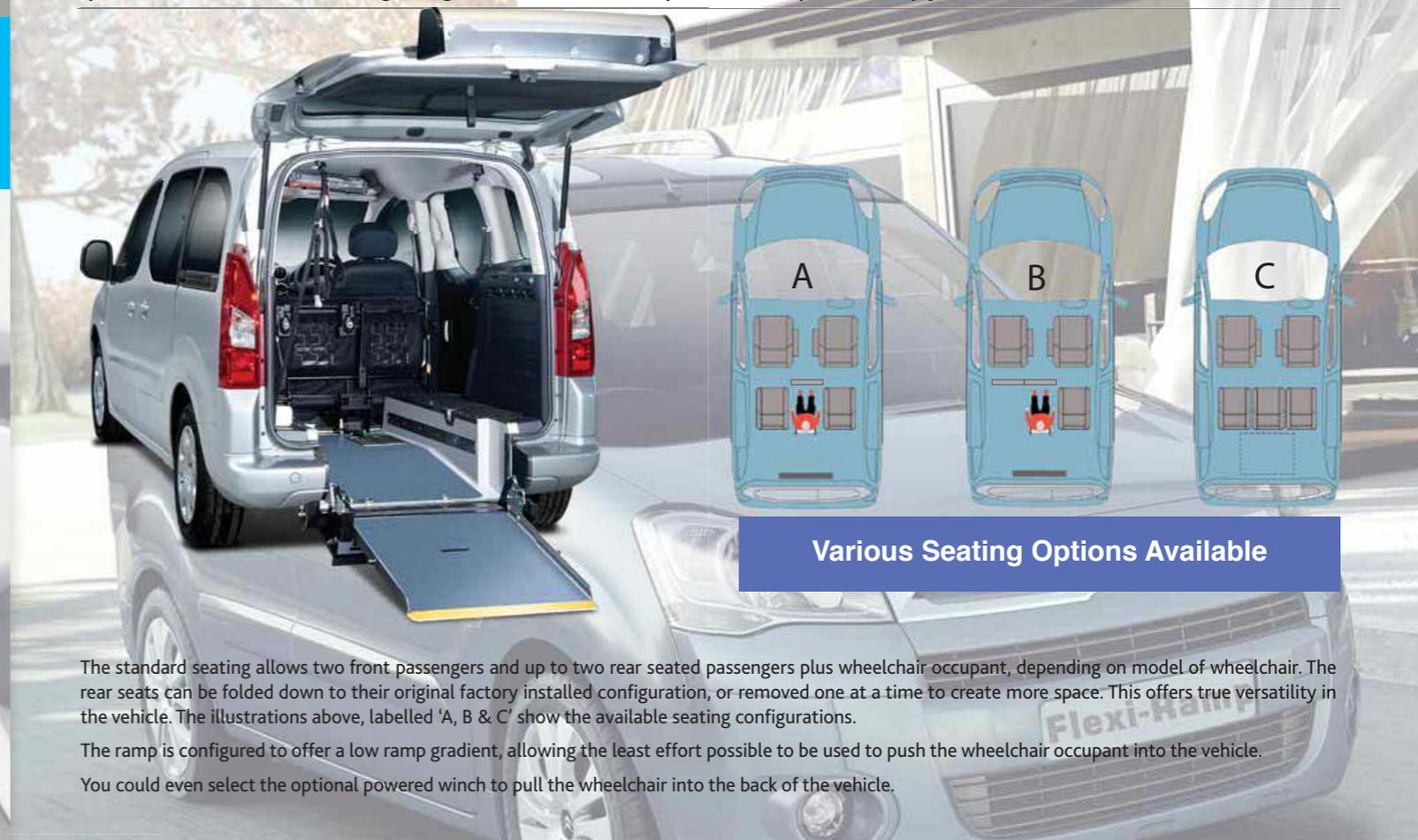
The standard seating allows two front passengers and up to two rear seated passengers plus wheelchair occupant, depending on model of wheelchair. The rear seats can be folded down to their original factory installed configuration, or removed one at a time to create more space. This offers true versatility in the vehicle. The illustrations above, labelled 'A, B & C' show the available seating configurations.
